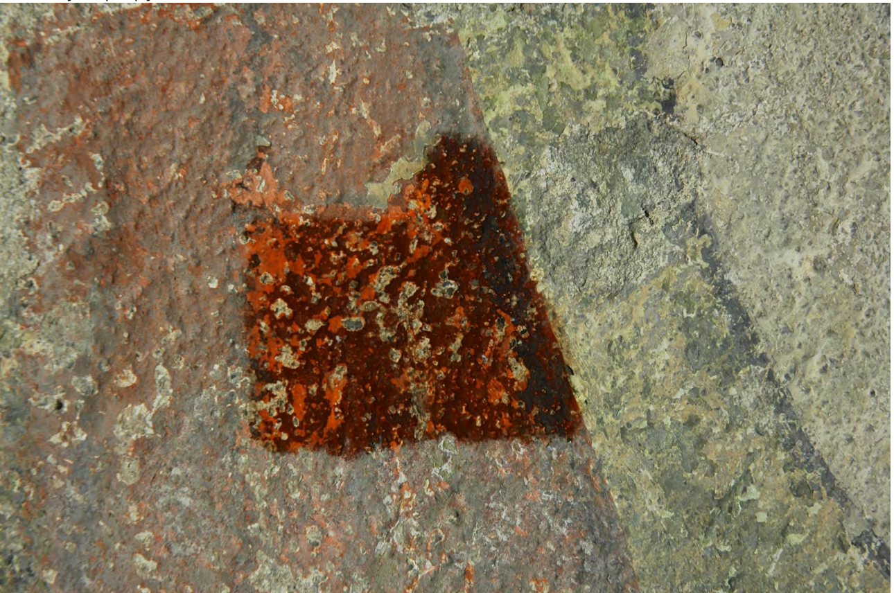
2 Hydropropylcellulose Klucel EF in Ethanol: 5%
